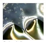
Cracks and splits after fusing.
