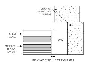
CROSS-SECTION OF DOUBLE-FIRE STACK
