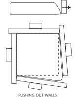
Uneven thickness most often is the result of a shelf that is not level. Be certain to level your shelf before you begin building on it, and then check the level after you have completed the stack.
