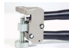
32 118 30 PROVETRO P-510 (für / for 3 - 16 mm Glas / glass) Dickglas Brechzange, 210 mm, 23 mm, Backenbreite, ummantelter Griff / Pliers for thick glass, 210 mm, 23 mm jaw width, coated grip
